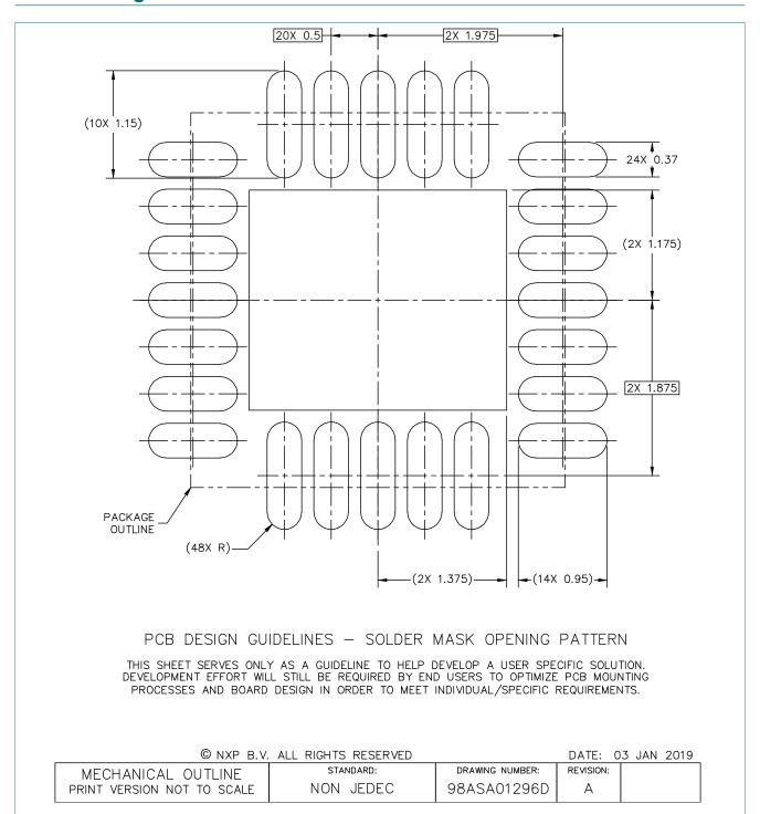
Figure 3. Reflow soldering footprint part1 for HTQFN24 (SOT1991-1(SC))
