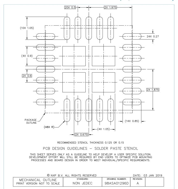
Figure 5. Reflow soldering footprint part3 for HTQFN24 (SOT1991-1(SC))
