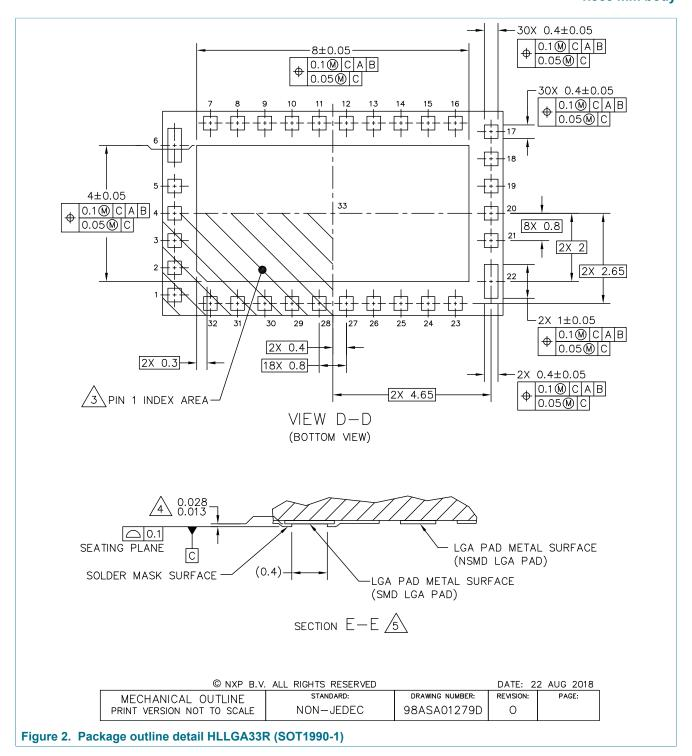
HLLGA33R, thermal enhanced low profile land grid array, 33 terminals, 0.8 mm pitch, 10 mm x 6 mm x 1.365 mm body
