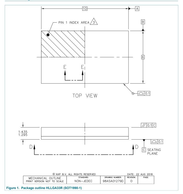
HLLGA33R, thermal enhanced low profile land grid array, 33 terminals, 0.8 mm pitch, 10 mm x 6 mm x 1.365 mm body
