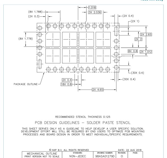
Figure 5. Reflow soldering footprint part3 for HLLGA33R (SOT1990-1)
