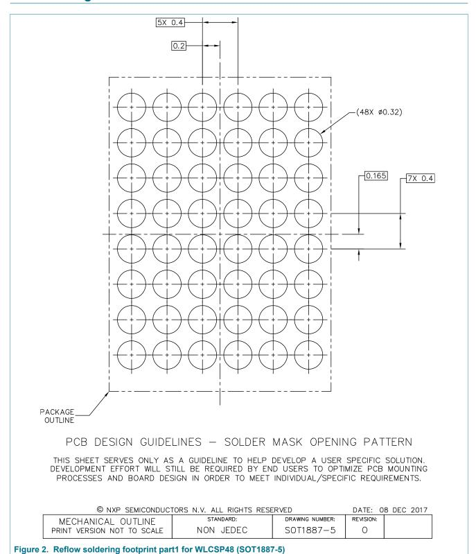
WLCSP48, wafer level chip-scale package; 48 bumps; 0.4 mm pitch, 2.51 mm x 3.55 mm x 0.525 mm body
