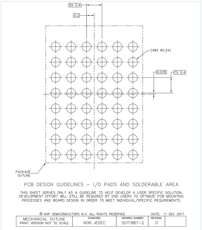
Fig. 4. Reflow soldering footprint part2 for WLCSP48 (SOT1887-2)
