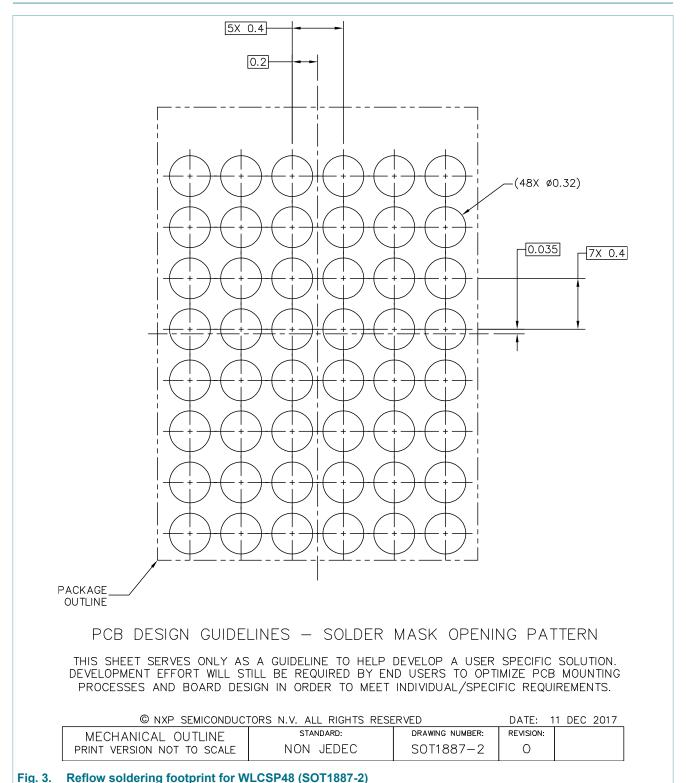
rig. 3. Renow soldering lootprint for WLCSP46 (SOT1667-2)
