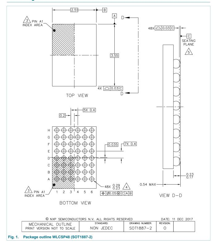
WLCSP48, wafer level chip-scale package; 48 bumps; 0.4 mm pitch, 2.51 mm x 3.55 mm x 0.5 mm body
