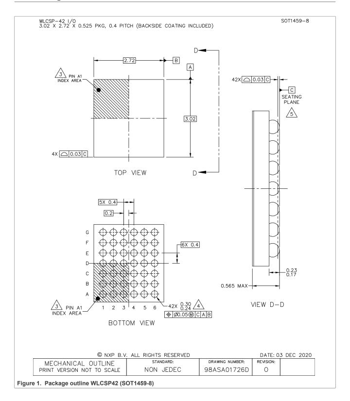
WLCSP42, wafer level chip scale package, 42 terminals, 0.4 mm pitch, 3.02 mm x 2.72 mm x 0.525 mm body (backside coating included)
