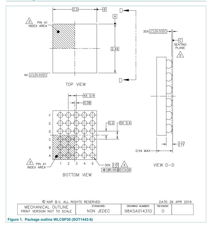
wafer level chip-scale package; 30 bumps; 0.4 mm pitch, 2.44 mm x 2.2 mm x 0.5 mm body (backside coating included)
