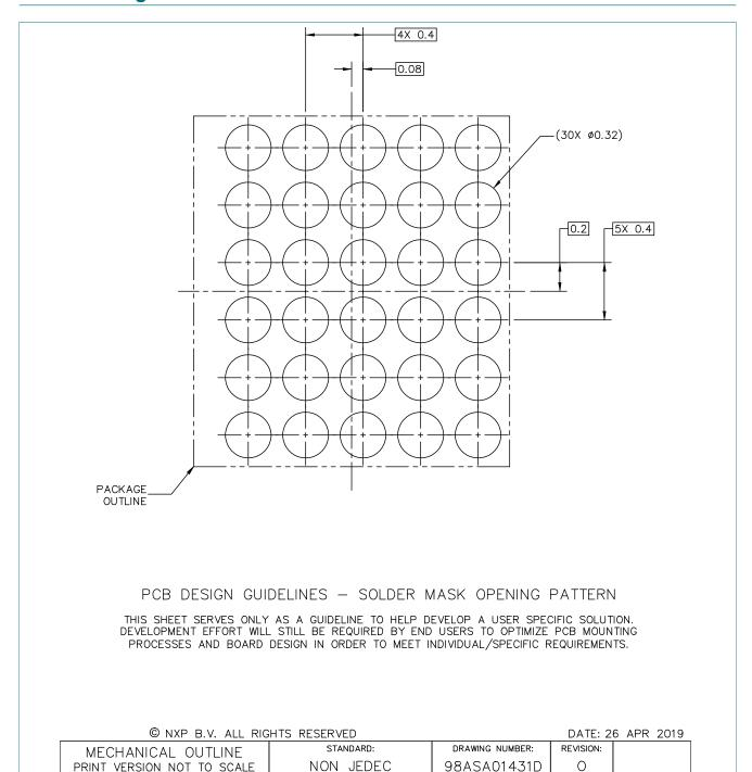
Figure 2. Reflow soldering footprint part1 for WLCSP30 (SOT1443-6)
