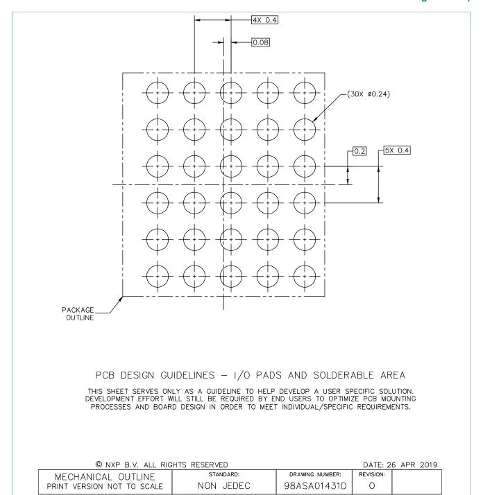
Figure 3. Reflow soldering footprint part2 for WLCSP30 (SOT1443-6)
