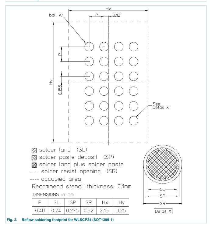
WLCSP24, wafer level chip-scale package; 24 bumps; 2.98 mm x 1.90 mm x 0.525 mm body (backside coating included)
