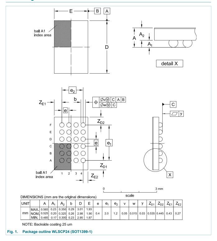
WLCSP24, wafer level chip-scale package; 24 bumps; 2.98 mm x 1.90 mm x 0.525 mm body (backside coating included)
