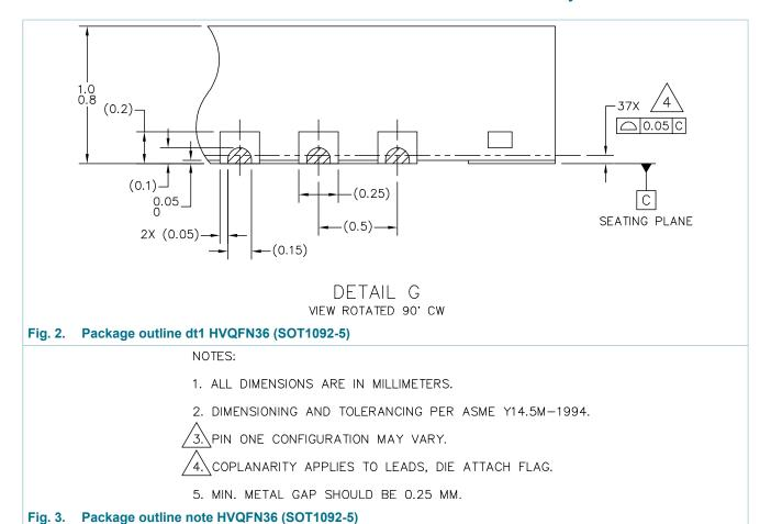
HVQFN36, plastic thermal enhanced very thin quad flat package; no leads, wettable flanks, 36 terminals; body 6 mm x 6 mm x 0.85 mm
