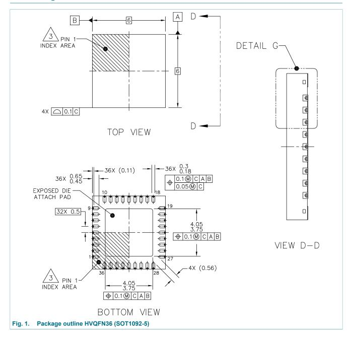
HVQFN36, plastic thermal enhanced very thin quad flat package; no leads, wettable flanks, 36 terminals; body 6 mm x 6 mm x 0.85 mm
