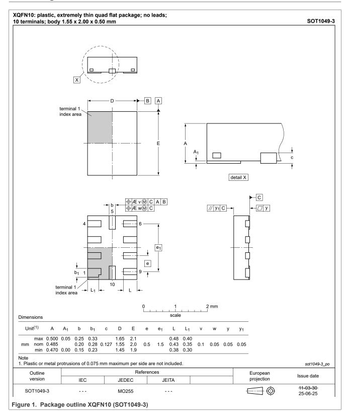
plastic, extremely thin quad flat package; 10 terminals; 0.5 mm pitch; 1.55 mm x 2 mm x 0.5 mm
