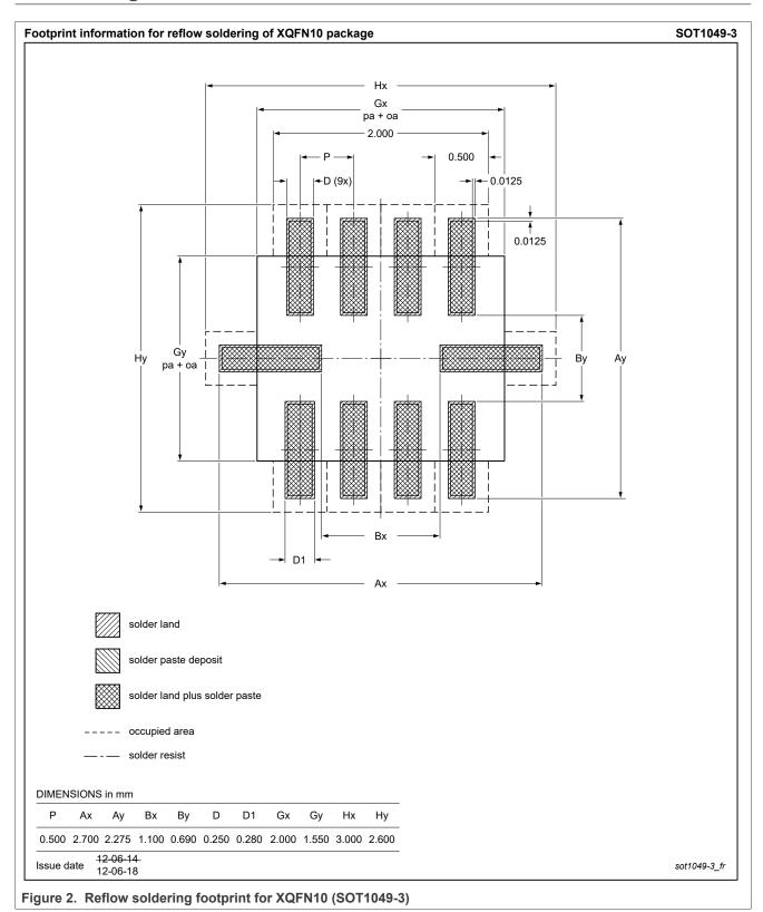
plastic, extremely thin quad flat package; 10 terminals; 0.5 mm pitch; 1.55 mm x 2 mm x 0.5 mm
