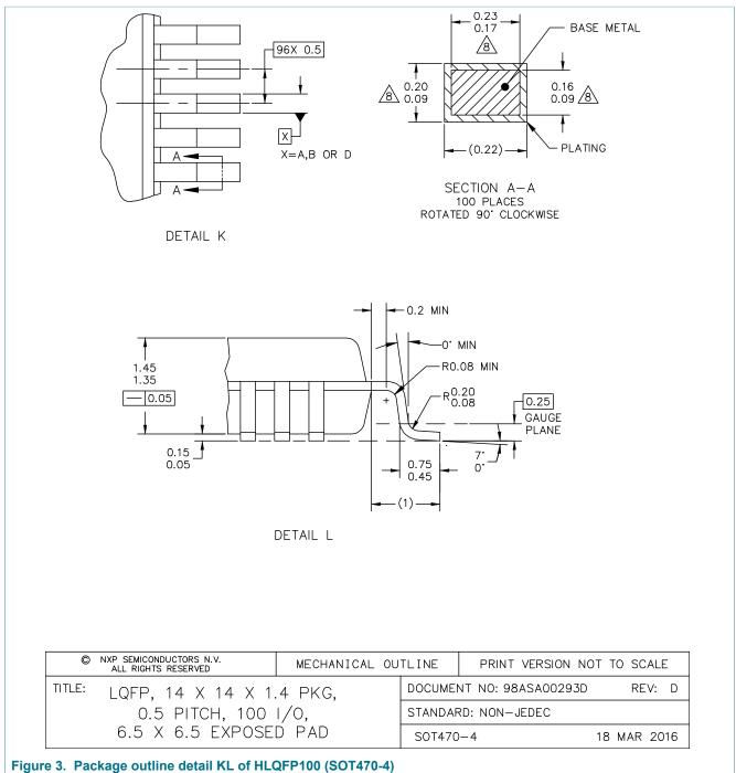
HLQFP100, plastic, thermal enhanced low profile quad flat package; 100 terminals; 0.5 mm pitch; 14 mm x 14 mm x 1.4 mm body
