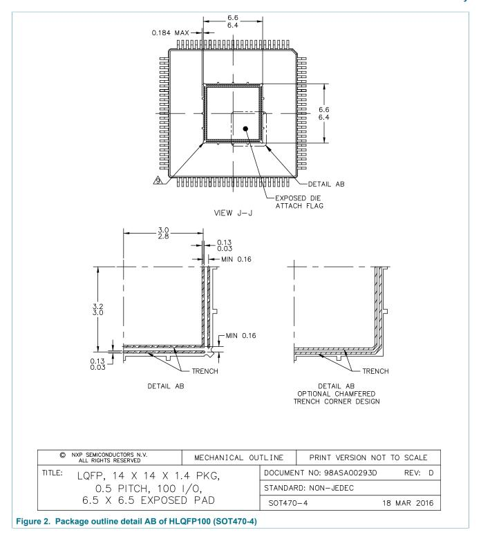
HLQFP100, plastic, thermal enhanced low profile quad flat package; 100 terminals; 0.5 mm pitch; 14 mm x 14 mm x 1.4 mm body
