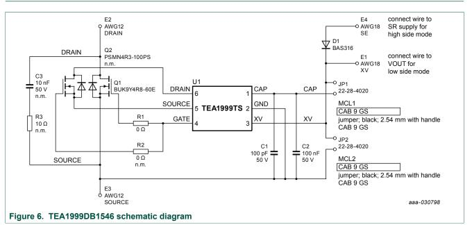
Figure 6 shows the schematic diagram of the TEA1999DB1546 demo board. The board incorporates the TEA1999TS controller and a 60 V logic-level power MOSFET. To facilitate easy connection for low-side, high-side, or self-supply applications, some adjustments have been made to the board:
