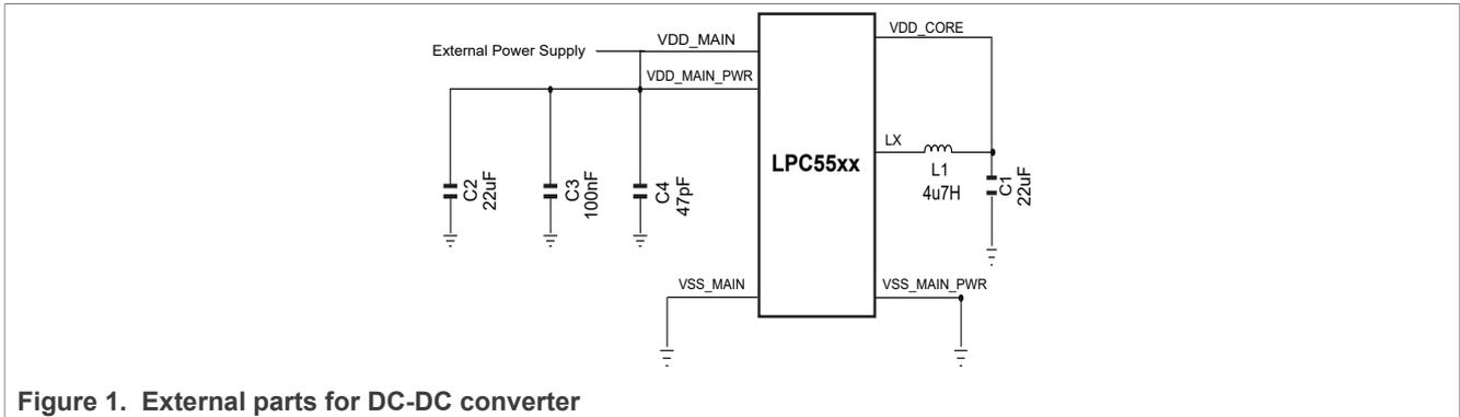
Figure 1. External parts for DC-DC converter
