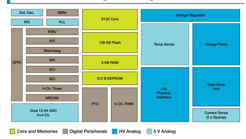
The MagniV MCUs offer the right blend of digital programmability and high-precision analog to streamline an automotive design. The S12ZVM product family integrates an MCU built on proven S12 technology, a voltage regulator, a LIN and CAN physical interface and a gate drive unit in order to control six external power MOSFETs.
