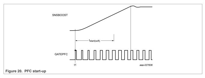
At t1, all conditions to start up the PFC are fulfilled. When the PFC starts switching, the maximum on-time is increased cycle-by-cycle from zero until the t<sub>on</sub> regulation limits the on-time of the PFC external MOSFET.
