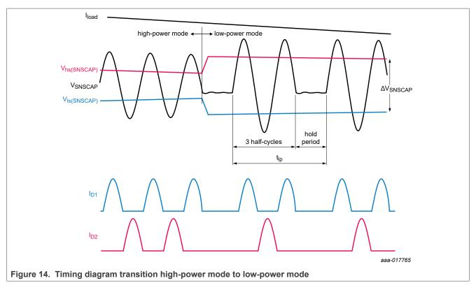
As the system continuously tracks the primary capacitor voltage, it knows exactly when to enter the "hold" period. It can also continue again at exactly the correct voltage and current levels of the resonant converter. In this way, a "hold" period can be introduced which reduces the magnetization and switching losses without any additional losses. The currents  $I_{D1}$  and  $I_{D2}$  (see <u>Figure 14</u>) are the secondary currents through diodes D1 and D2 (see <u>Figure 25</u>).
