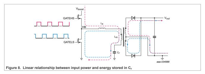
When the high-side switch is on, a primary current is flowing through the transformer and resonant capacitor  $C_r$  as indicated by the red line. Half the energy the input delivers is transferred to the output. The other half charges resonant capacitor  $C_r$ . The voltage across the resonant capacitor increases.
