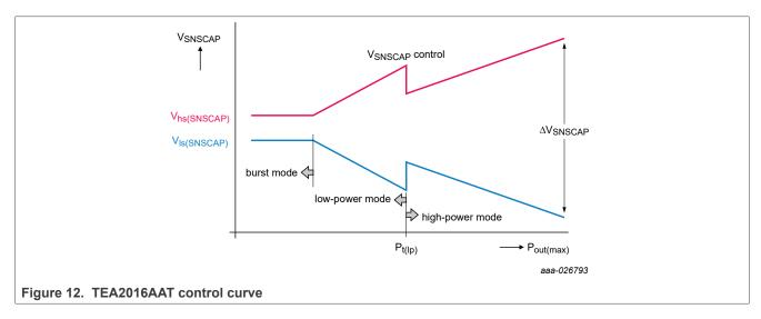
When the output power ( $P_{out}$ ) is at its maximum, the low capacitor voltage level ( $V_{Is(SNSCAP)}$ ) is at its minimum, and the high capacitor voltage ( $V_{hs(SNSCAP)}$ ) is at its maximum level. According to Equation 1 in Section 8.2, the maximum  $\Delta V_{SNSCAP}$  ( $V_{hs(SNSCAP)} - V_{Is(SNSCAP)}$ ), which is the divided  $\Delta V_{Cr}$  voltage, corresponds to the maximum output power.
