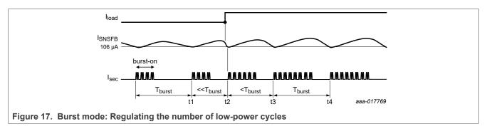
The system continuously measures the burst period from the start of the previous burst-on period to a new burst-on period. At t1, the measured burst period ( $t_{burst}$ ) equals the required  $T_{burst}$ . So, the next number of low-power cycles equals the number of previous low-power cycles. At a constant output power, the system expects that when the next burst-on period has the same number of low-power cycles as the previous burst-on period, the burst period ( $T_{burst}$ ) remains constant.
