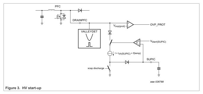
The maximum current of the internal current source is limited to  $I_{ch(SUPIC)}$ . To limit the IC dissipation, the charge current is reduced when the current source exceeds its maximum temperature ( $T_{SUPICcharger}$ ).
