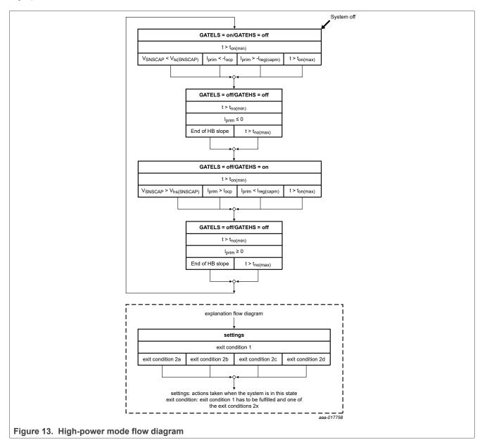
Initially, GATELS is on and GATEHS is off. The external bootstrap buffer capacitor ( $C_{SUPHS}$ ) is charged via the GATELS pin and an external diode. The system remains in this state for at least the minimum on-time ( $t_{on(min)}$ ) of GATELS. Before entering the next state, one of the following conditions must be fulfilled:
