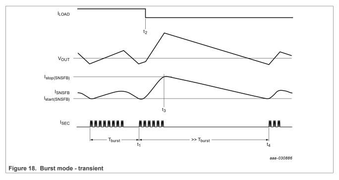
At t1, the system starts with a new burst cycle period. Shortly later at t2, the output load is reduced. As a result the output voltage shows an overshoot and the optocoupler current increases. To limit the overshoot, the system also ends the burst cycle when the optocoupler current exceeds the I<sub>ston/burst</sub>) level.
