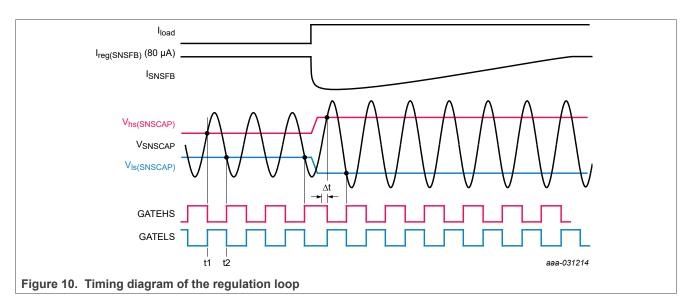
When the divided resonant capacitor voltage ( $V_{SNSCAP}$ ) exceeds the capacitor voltage high level ( $V_{hs(SNSCAP)}$ ), the high-side MOSFET is switched off (see <u>Figure 10</u> (t1)). After a short delay, the low-side MOSFET is switched on. Because of the resonant current, the resonant capacitor voltage initially increases further but eventually drops.
