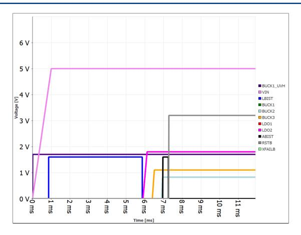
The signals depicted above are enable signals for each regulator. They don't represent the actual ramp voltage.
