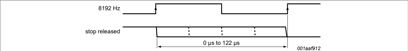
Figure 6. ST bit release timing
