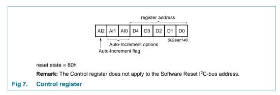
When the Auto-Increment flag is set (AI2 = 1), the five low order bits of the Control register are automatically incremented after a read or write. This allows the user to program the registers sequentially. Four different types of Auto-Increment are possible, depending on AI1 and AI0 values.
