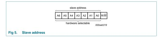
The last bit of the address byte defines the operation to be performed. When set to logic 1 a read is selected, while a logic 0 selects a write operation.
