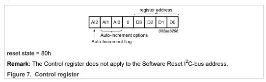
When the Auto-Increment flag is set (AI2 = 1), the four low order bits of the Control register are automatically incremented after a read or write. This allows the user to program the registers sequentially. Four different types of Auto-Increment are possible, depending on AI1 and AI0 values.
