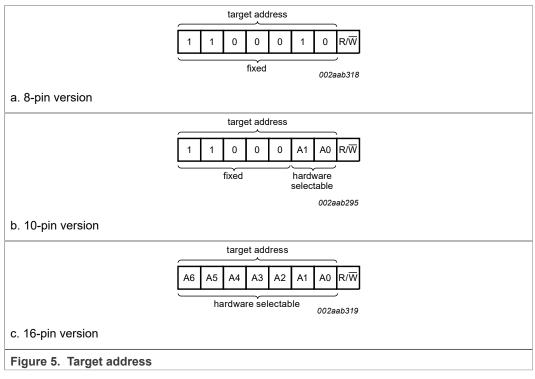
The last bit of the address byte defines the operation to be performed. When set to logic 1 a read is selected, while a logic 0 selects a write operation.
