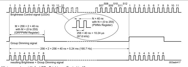
Minimum pulse width for LEDn Brightness Control is 40 ns.
