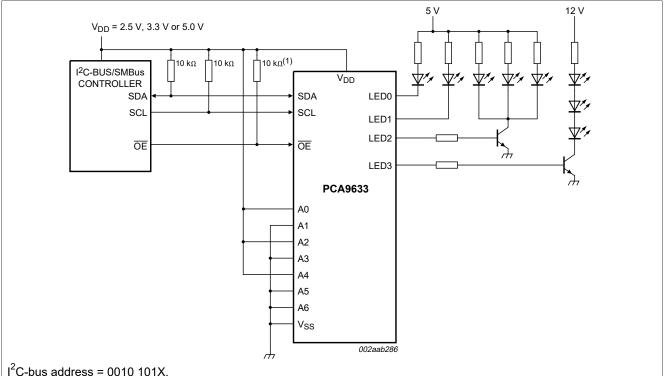
All of the 4 LEDn outputs configurable as either open-drain or totem pole. Mixing of configurations is not possible.
