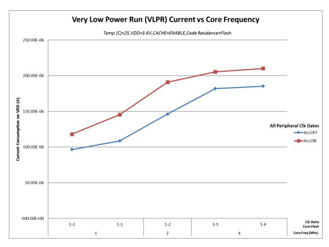
Figure 5. VLPR mode current vs. core frequency
