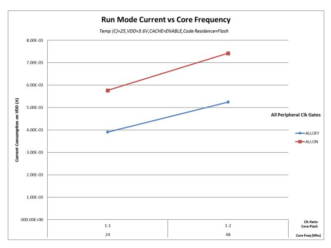
Figure 4. Run mode supply current vs. core frequency
