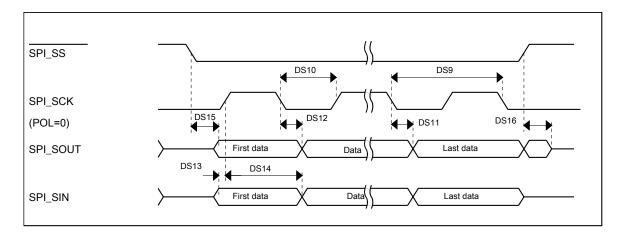
Figure 13. DSPI classic SPI timing — slave mode
