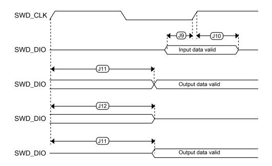
Figure 7. Serial wire data timing
