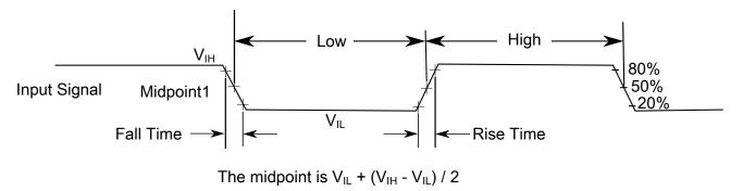
Figure 3. Input signal measurement reference
