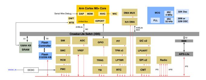
Figure 2. MWCT1R24ZVHT Detailed Block Diagram
