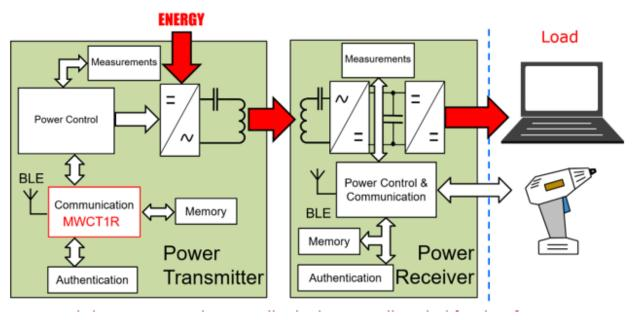
Figure 1. Wireless charging system-functional diagram
