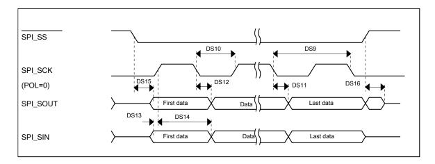
Figure 11. DSPI classic SPI timing — slave mode
