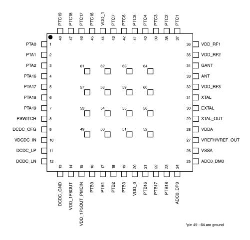
Figure 15. 48-pin Laminate QFN pinout diagram
