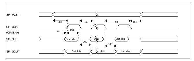
Figure 10. DSPI classic SPI timing — master mode
