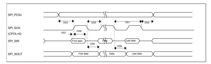
Figure 12. DSPI classic SPI timing — master mode
