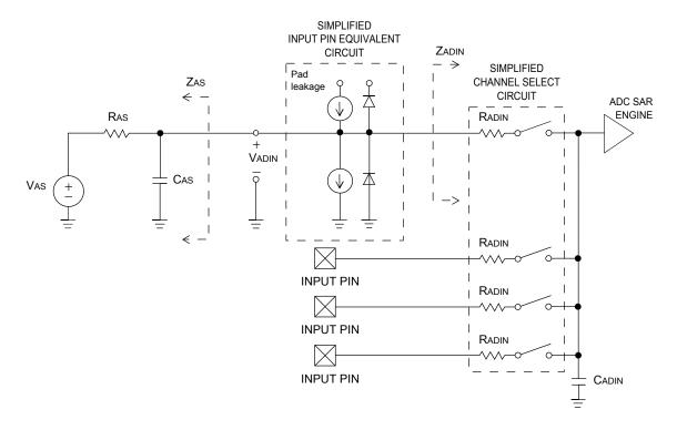
Figure 9. ADC input impedance equivalency diagram
