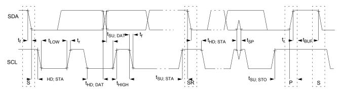
Figure 14. Timing definition for fast and standard mode devices on the I<sup>2</sup>C bus
