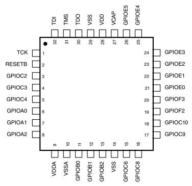
Figure 26. 32-pin LQFP and QFN
