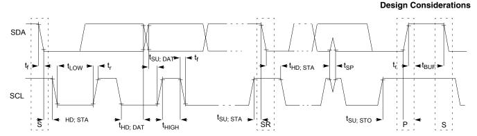
Figure 21. Timing definition for fast and standard mode devices on the I<sup>2</sup>C bus
