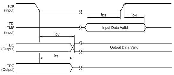
Figure 7. Test access port timing diagram
