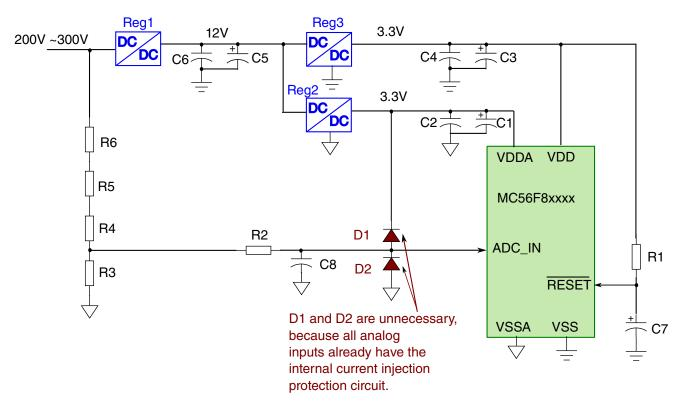
Figure 22. Protection Circuit Example
