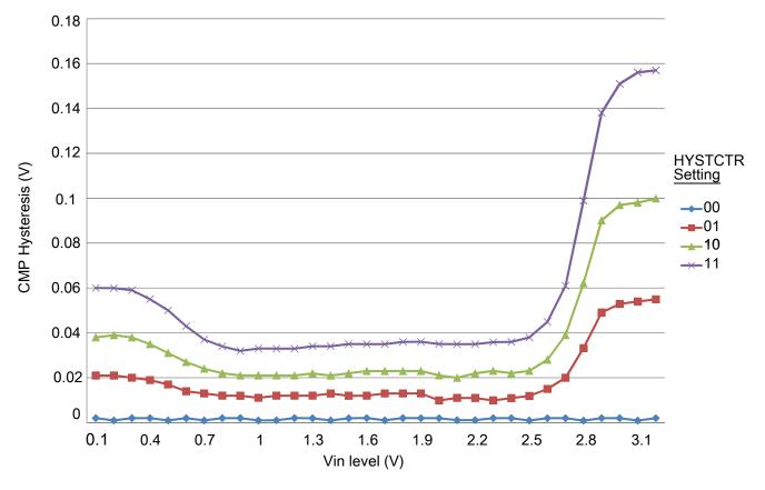
Figure 12. Typical hysteresis vs. Vin level (V<sub>DD</sub> = 3.3 V, PMODE = 1)
