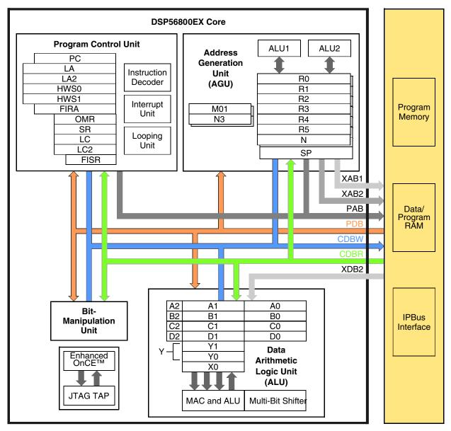
Figure 1. 56800EX basic block diagram
