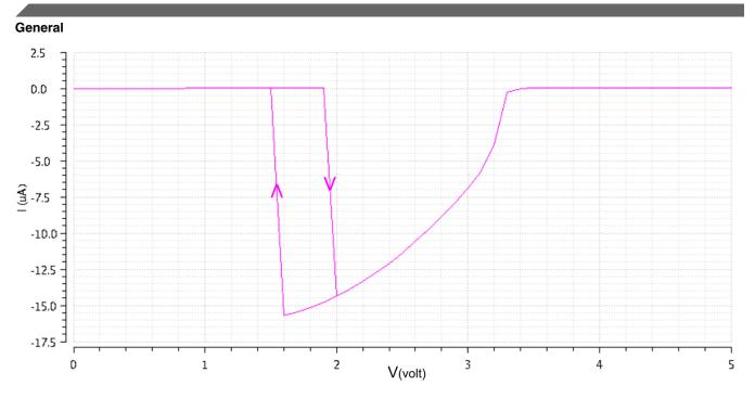
Figure 5.  $I_{IN}/I_{OZ}$  vs.  $V_{IN}$  (typical; pull-up disabled) (design simulation)
