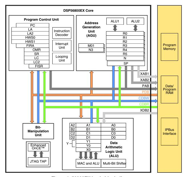
Figure 1. 56800EX basic block diagram
