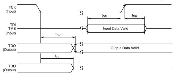
Figure 7. Test access port timing diagram
