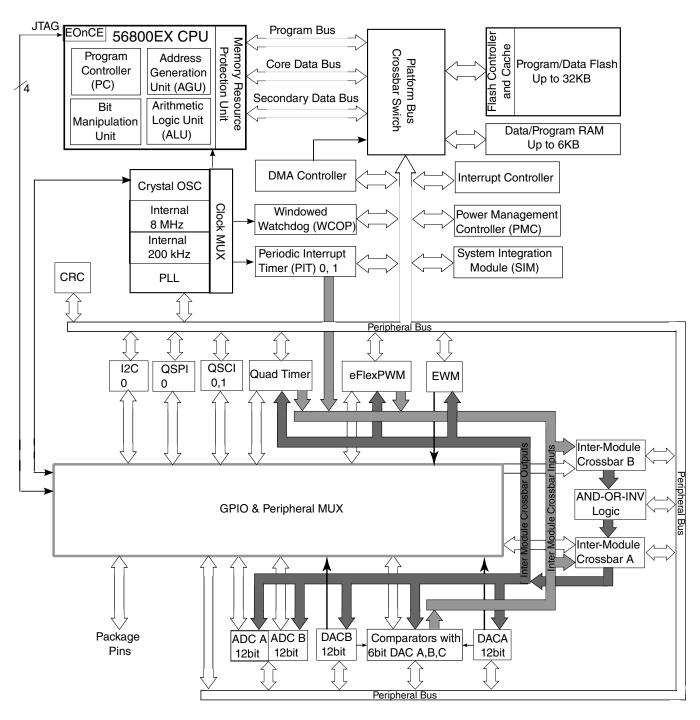
Figure 2. System diagram
