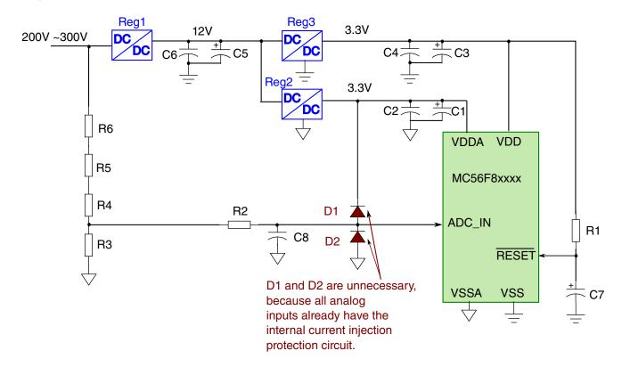
Figure 22. Protection Circuit Example
