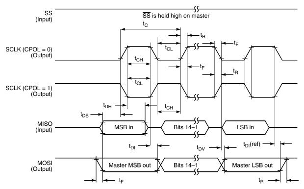
Figure 14. SPI master timing (CPHA = 0)
