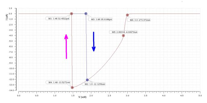
Figure 5. I<sub>IN</sub>/I<sub>OZ</sub> vs. V<sub>IN</sub> (typical; pull-up disabled) (design simulation)
