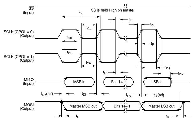
Figure 15. SPI master timing (CPHA = 1)
