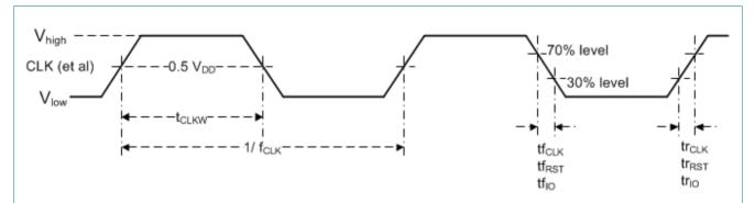
Fig 11. External clock drive and AC test timing reference points of I2C\_SDA, I2C\_SCL, and RST\_N (see <u>Table note [3]</u> and <u>Table note [4]</u>) in open drain mode
