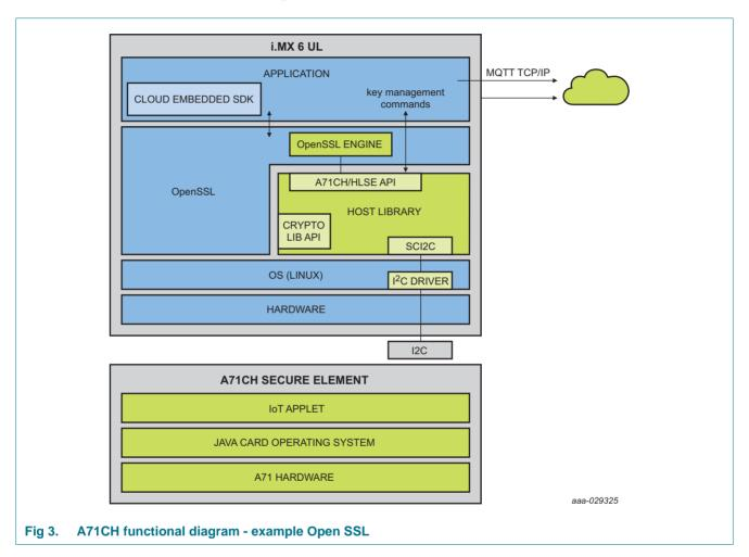
The A71CH uses I<sup>2</sup>C as communication interface as described in the following section. The A71CH commands are wrapped using the Smartcard I<sup>2</sup> protocol (SCI2C). The detailed documentation for the A71CH commands [ref to APDU Spec] and SCI2C encapsulation (Ref. 3) is available in NXP docstore."
