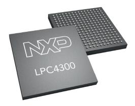
NXP 204 MHz, 32-bit Cortex-M4 /Cortex-M0 DSC LPC4300 series
