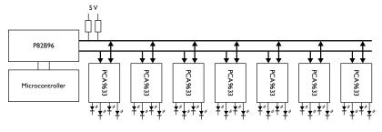
The PCA9633 demo board configured in Multiple-card Chase Mode (Mode 5)
