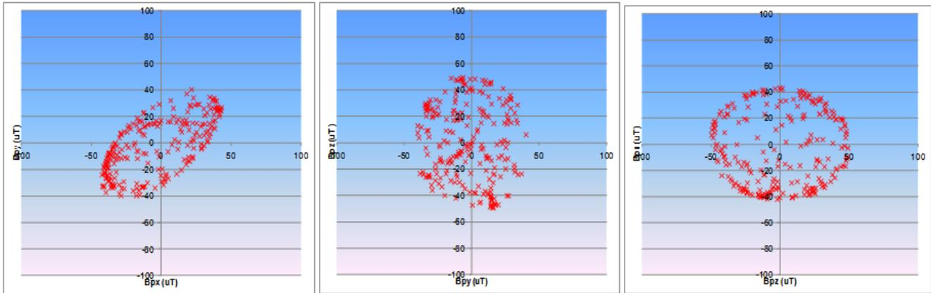
**Figure 5. Measured magnetometer locus - hard-iron correction applied**
