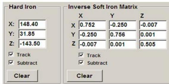
Figure 4. Calibration coefficients computed by the RD4247MAG3110 software
