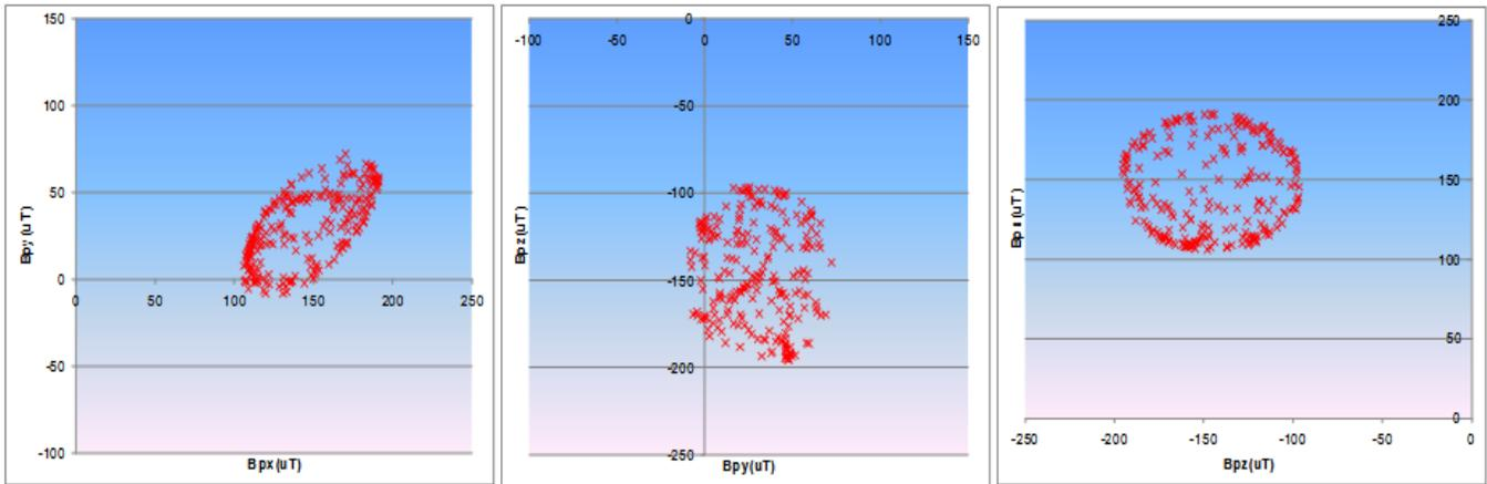
Figure 3. Measured magnetometer locus - no correction applied
