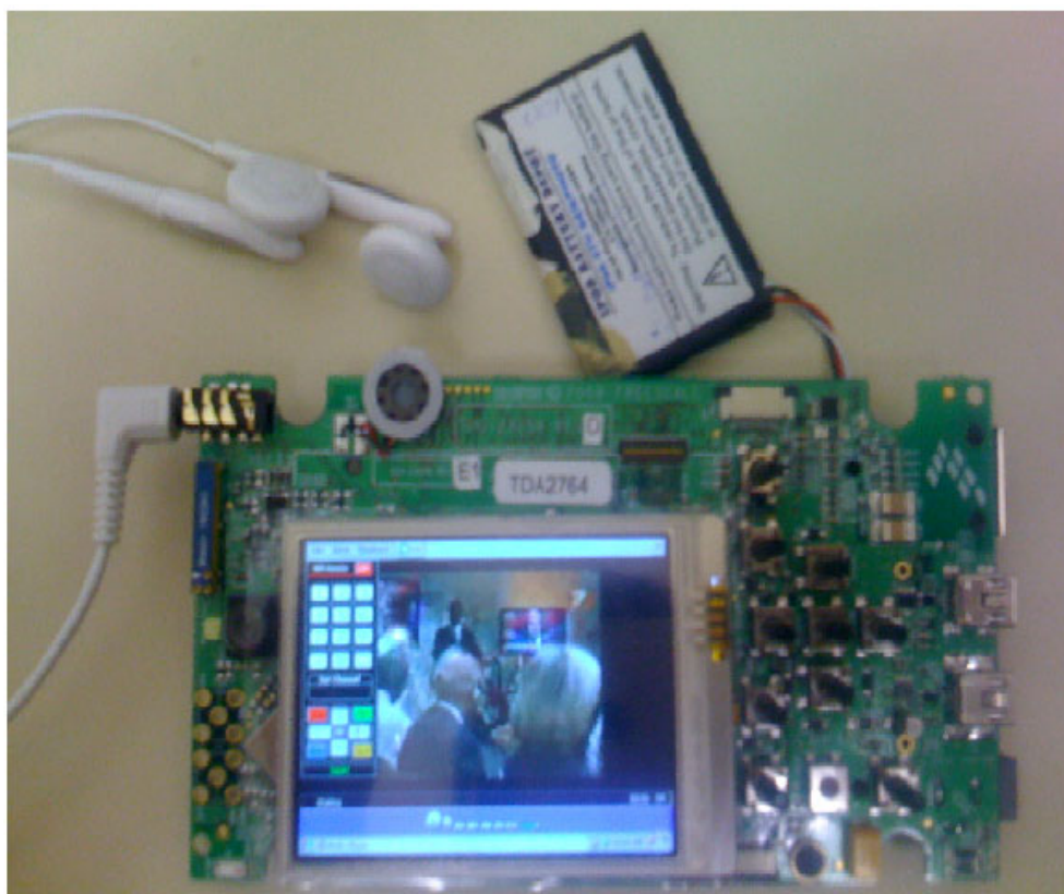
Figure 8. i.MX31 PDK Displaying Video from Server
