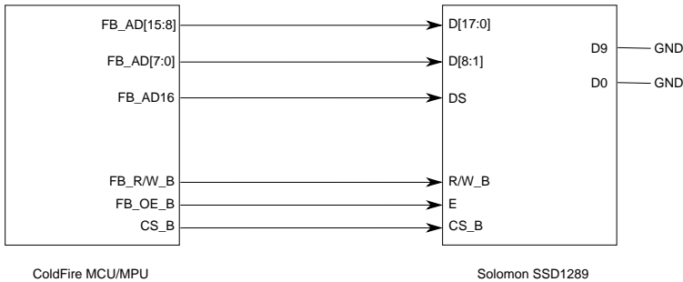
Figure 5. 16-bit bus interface to ColdFire MCU/MPU
