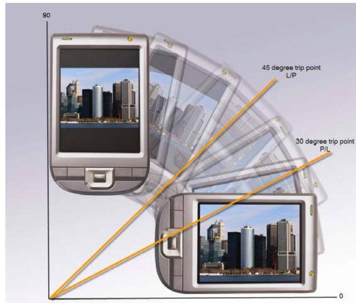
**Figure 5. Built-in Detection Trip Point for L/P and 30 Degree for P/L**
