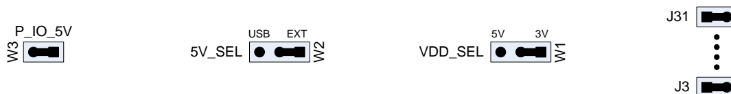
Figure 6. DEMO9S08AW60 Jumper Settings
