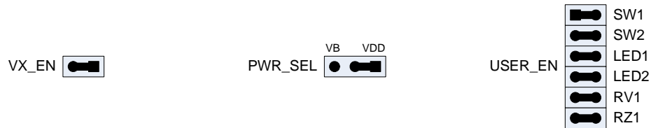
Figure 5. DEMO9S08QG8 Jumper Settings
