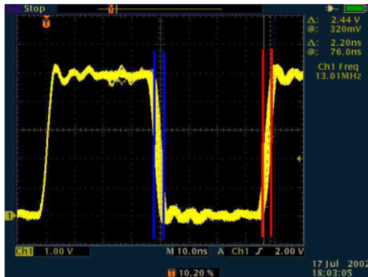
Figure 1. Typical Internal Oscillator Output
