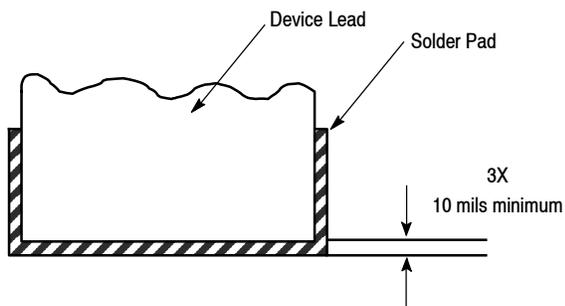
**Figure 6. Pad Size in Relation to the Lead**
