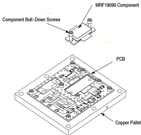
Figure 2. MRF19090 90-Watt Power Device Board Construction
