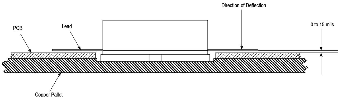
**Figure 4. Direction of the Lead Deflection**
