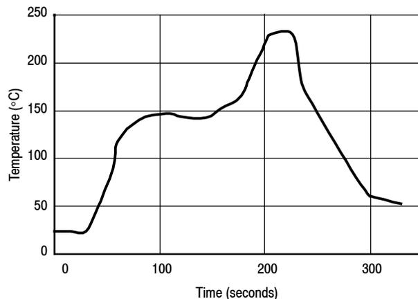
**Figure 7. Typical Solder Reflow Profile for Sn/Pb/Ag Solder**
