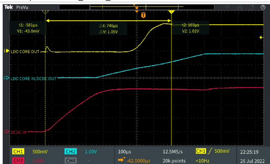
Figure 9. LDO core startup time
