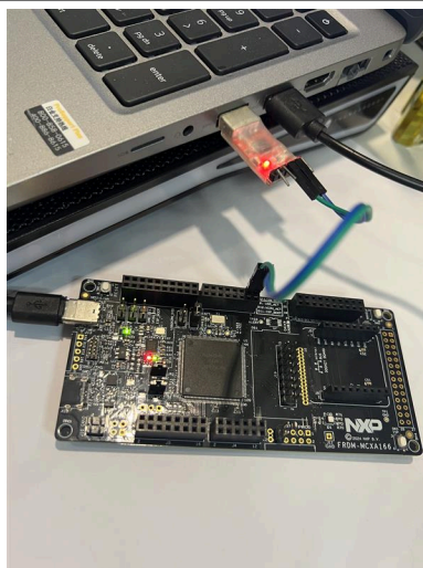
Figure 4. The FRDM-MCXA346 board connects with the PC through a USB-to-LPUART dongle
