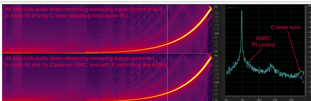
Figure 8. USB audio down streaming 48 kHz synchronized by CTimer and ASRC
