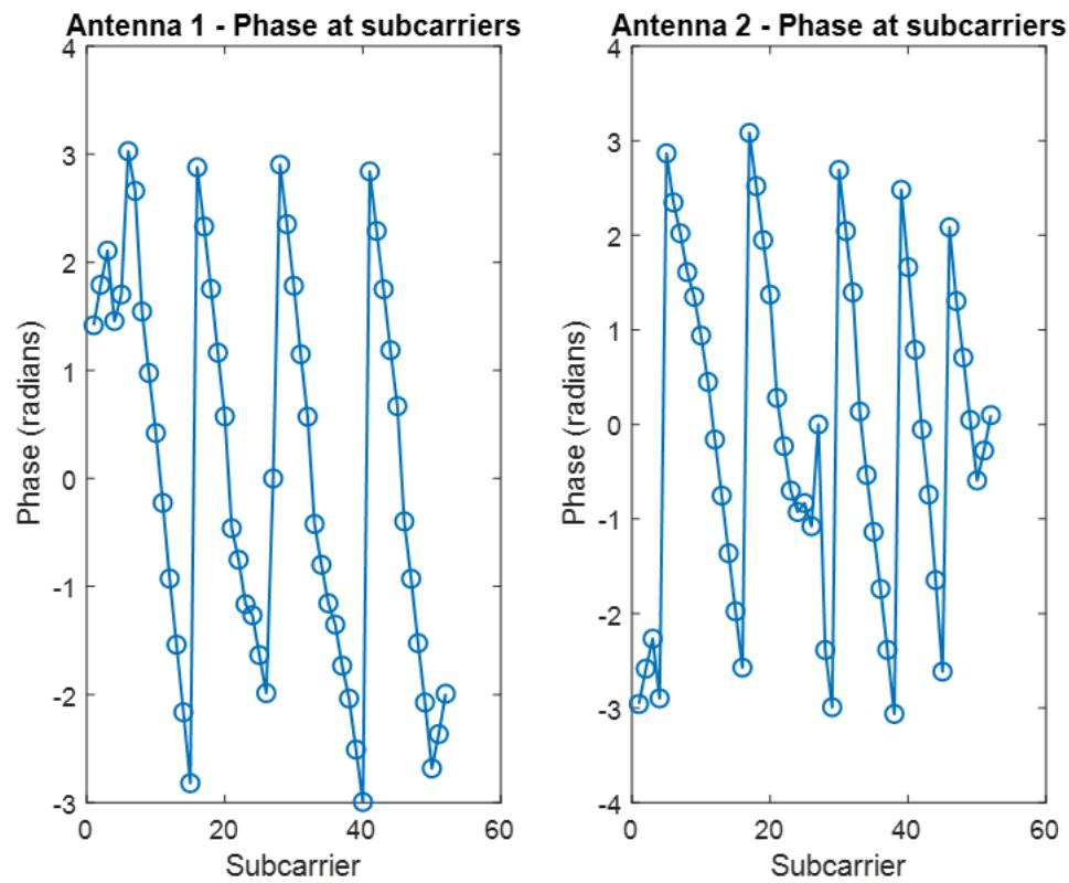
Figure 4. Phase across reported subcarriers for receive antennas
