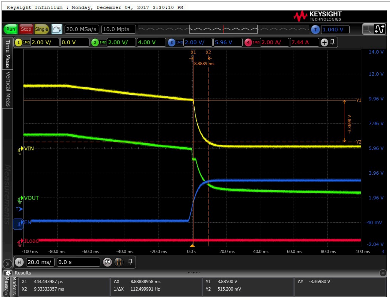
Figure 7. VBUS pin going down below Vsafe0V and Vsafe5V after VBUS detached and switch disabled. Maximum 650ms below Vsafe0V, and Maximum 275ms below Vsafe5V
