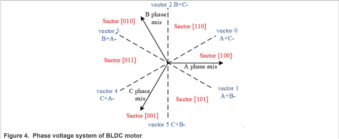
Figure 4. Phase voltage system of BLDC motor
