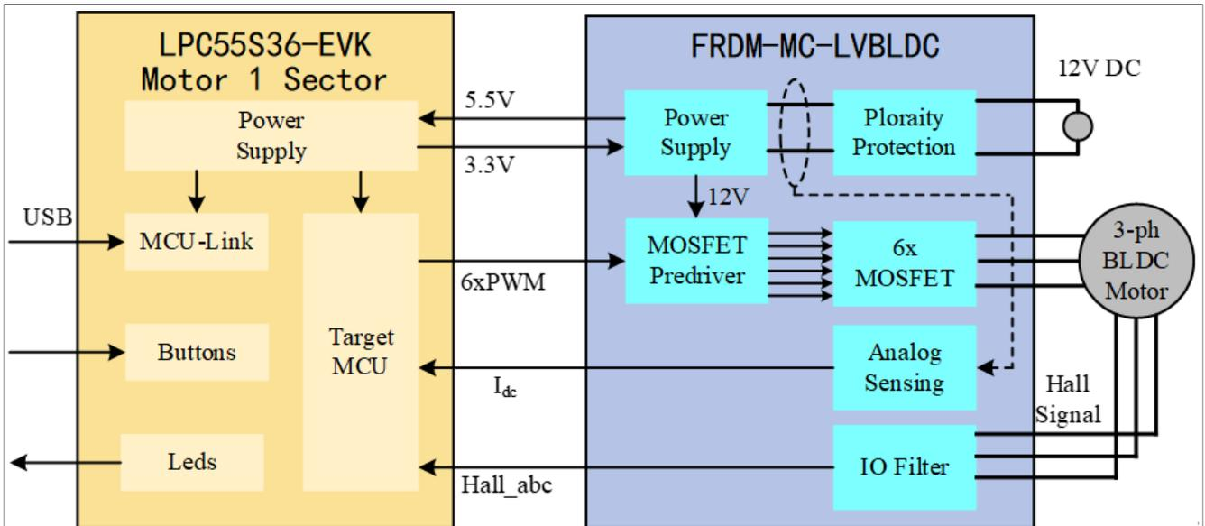
Figure 5. Motor control development platform block diagram
