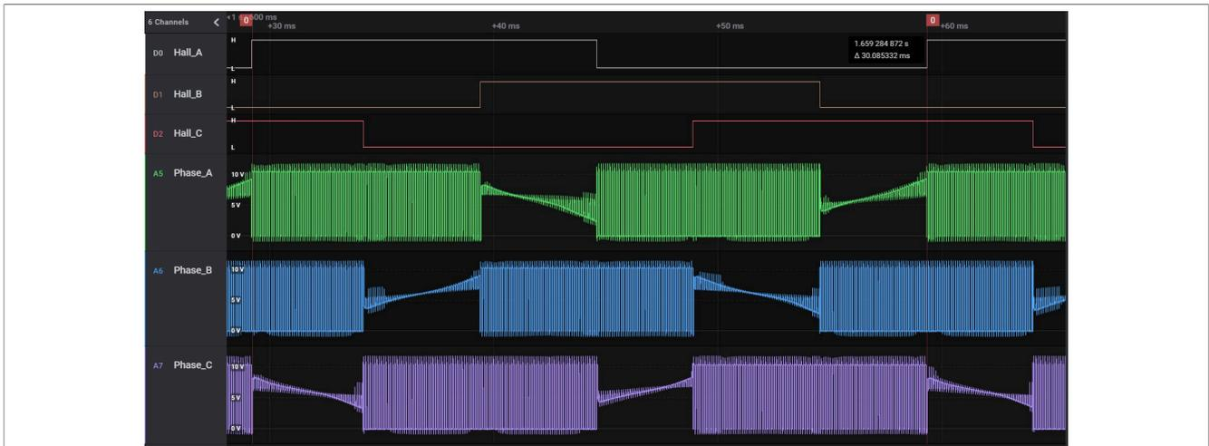
Figure 11. Hall signal and motor-winding terminal at 1000 rpm
