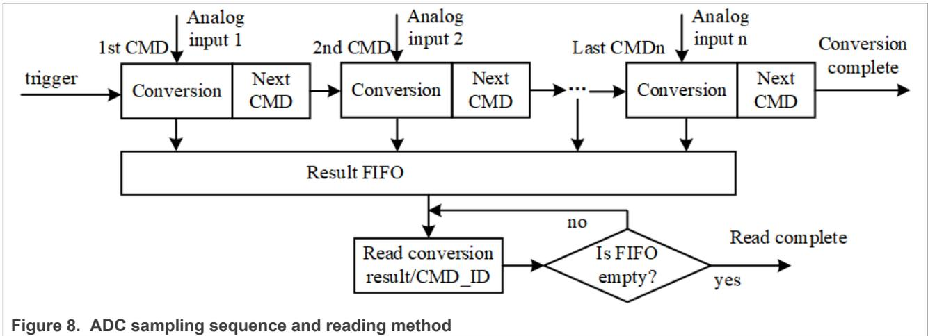
Figure 8. ADC sampling sequence and reading method
