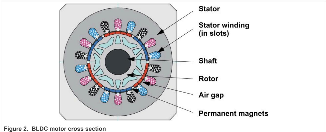
The Hall sensor is installed on the axis of the stator three-phase winding to detect the rotor position.
