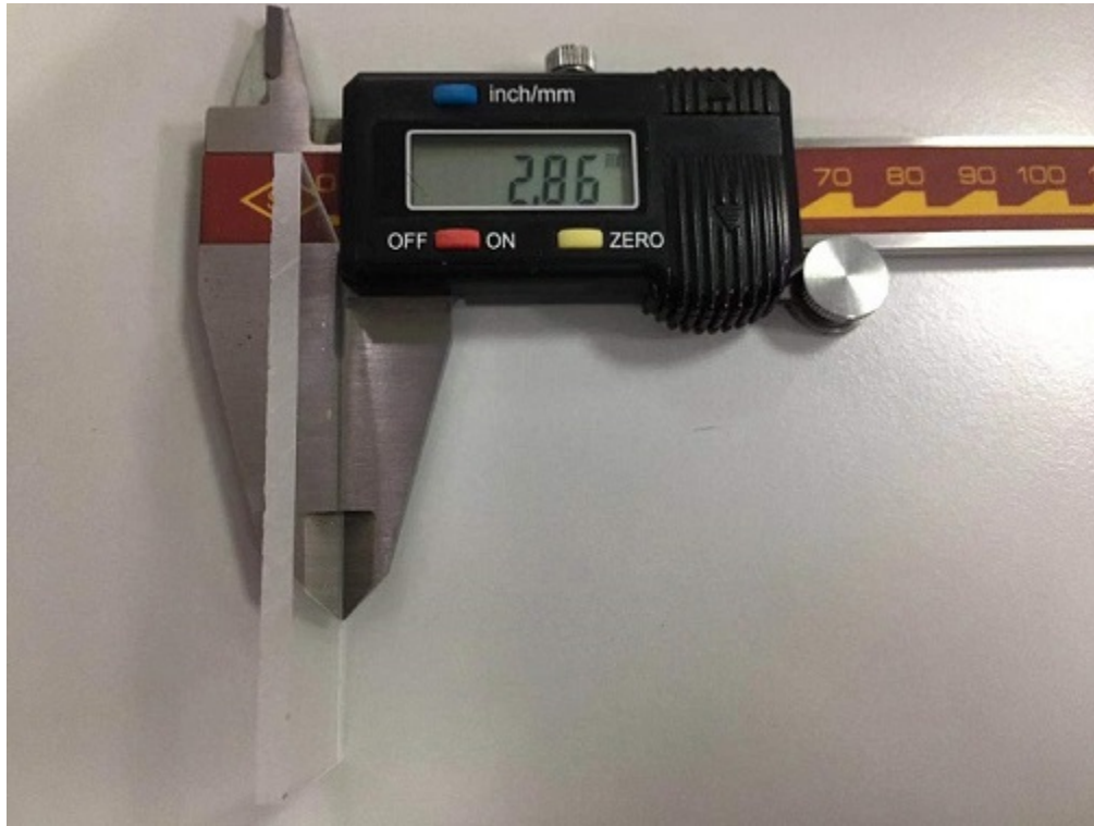
Figure 4. Use acrylic board with 3 mm thickness
