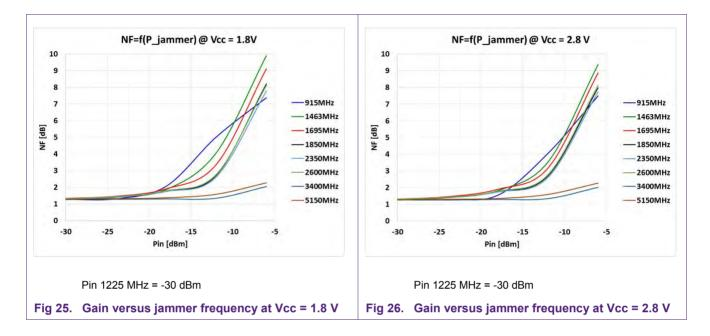
The figures below show the noise figure (NF) related to the jamming frequency at different voltage supplies. The influence of the jammer decreases as the frequency separation between the L2-band and the jammer increases.
