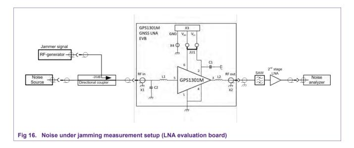
With the results of these measurements and the specification of the SAW filter, the jammer power levels that cause noise increase can be calculated.
