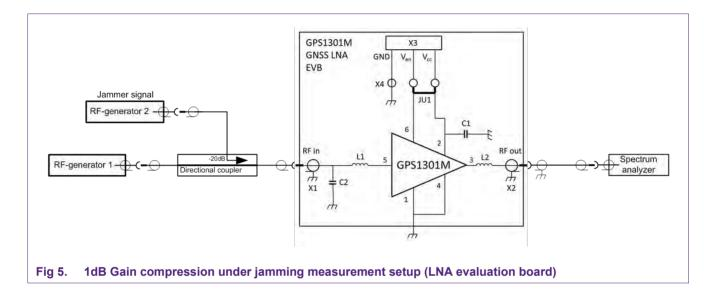
The gain of the DUT was measured between port RFin and RFout of the EVB at the GNSS frequency 1225 MHz, while simultaneously a jammer power signal was swept at the 20dB attenuated input port of the Directional Coupler. Please note that the drive power of the jammer is 20 dB lower at the input of the DUT caused by the directional coupler.
