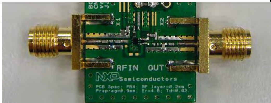
Fig 4. Printed circuit board of the BGF7003 2.62 ~ 2.69GHz evaluation board
