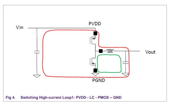
To minimize electromagnetic interference (EMI), it is essential to minimize the length and area of the switching high current loops. It is also critical that the two switching current paths are matched as closely as possible.
