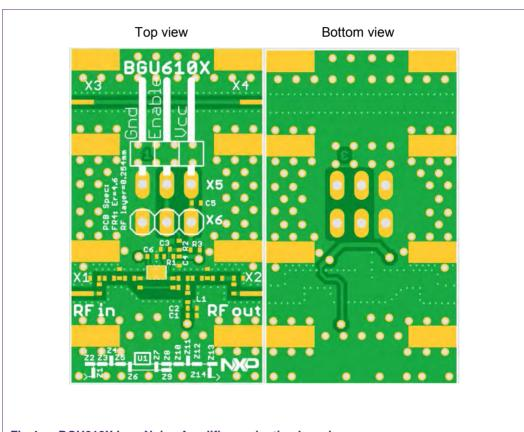
Fig 4. BGU610X Low Noise Amplifier evaluation board
