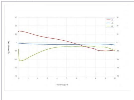
Fig 6. S-Parameters up to 10 GHz, Vcc=3.0V, Icc=3.1mA
