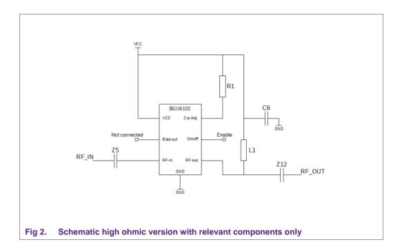
At the position of L1 a resistor is placed. To accomplish a higher gain, one may replace this resistor by a coil with the result of a higher gain but a smaller useable bandwidth.
