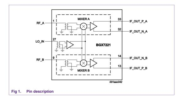
Each mixer, A and B employs a transformer to convert the single-ended RF input into a differential signal to drive the passive MOS mixer. The MOS mixer directly drives the IF amplifier. Its open-collector outputs deliver the differential signal into an external transformer load, referenced to the 5 V supply for maximum signal swing. Each mixer can be independently powered-off by a combination of POFF\_1 and POFF\_2.
