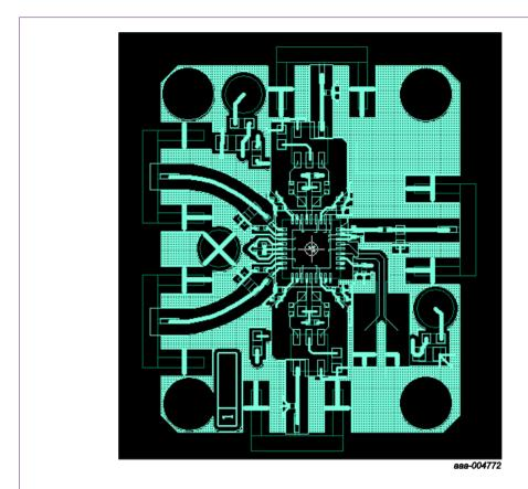
Fig 5. Evaluation board top layer PCB layout
