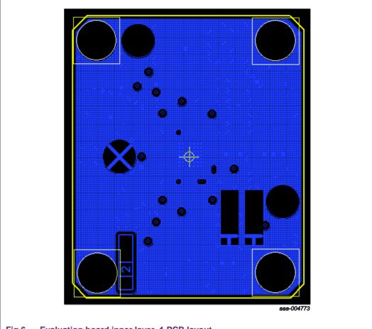
Fig 6. Evaluation board inner layer\_1 PCB layout
