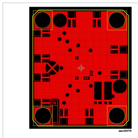
Fig 8. Evaluation board bottom layer PCB layout
