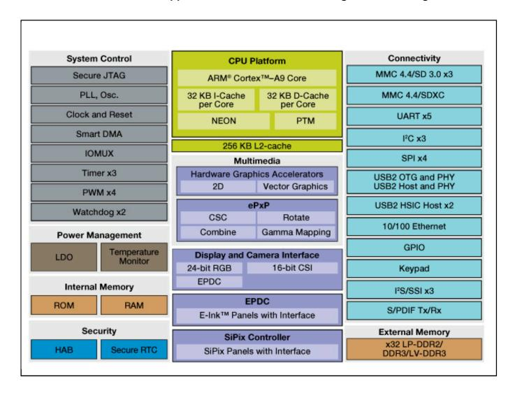
View additional information for i.MX 6SoloLite Processors - Single-Core, Low-Power, EPD Controller, Arm® Cortex®-A9 Core.
