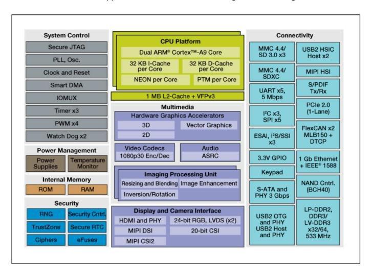
View additional information for i.MX 6Dual Processors - Dual-Core, 3D Graphics, HD Video, Multimedia, Arm® Cortex®-A9 Core.
