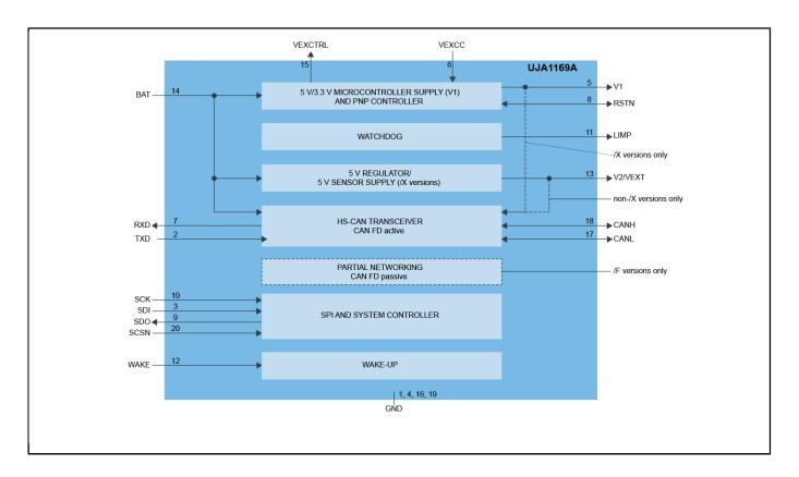
View additional information for Mini High-Speed CAN System Basis Chip.
