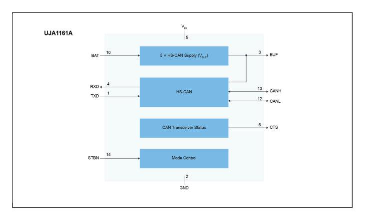
View additional information for Self-Supplied High-Speed CAN Transceiver with Standby Mode.
