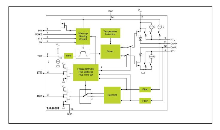
View additional information for Fault-Tolerant CAN Transceiver.
