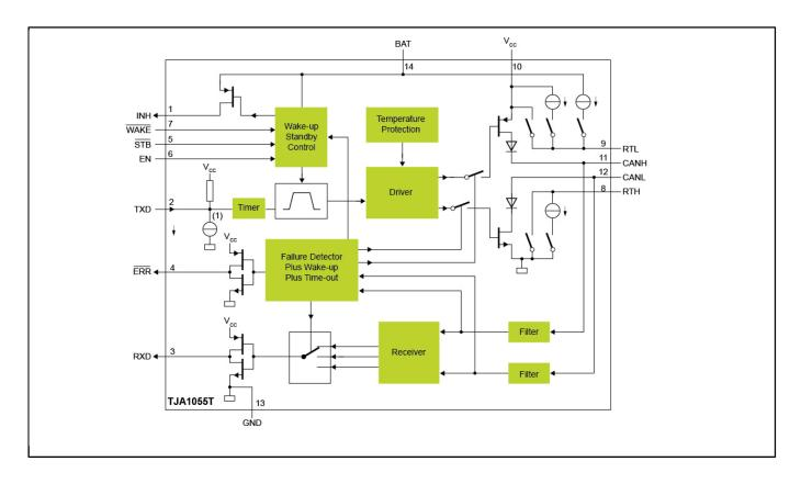
View additional information for Fault-Tolerant CAN Transceiver.
