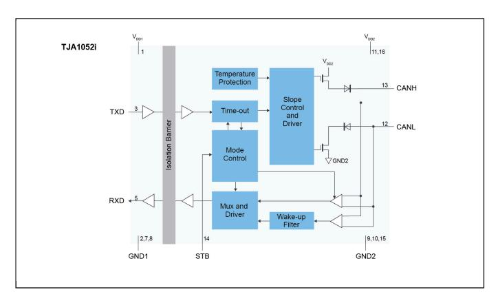
View additional information for Galvanically-Isolated High-Speed CAN Transceiver.
