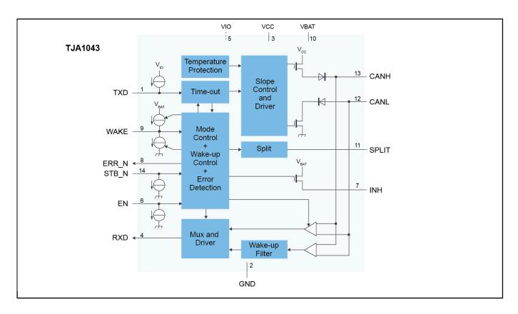
View additional information for High-Speed CAN Transceiver with Standby and Sleep Mode.
